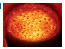
Breaking the coke habit: By coupling thermal decomposition with catalytic partial oxidation, an effective method has been developed to convert solid biomass such as cellulose into synthesis gas (see photo of a hot Rh catalyst surface). Not only is the process fast (< 70 ms), it also avoids the formation of coke, which is known to deactivate catalyst surface sites and block surface reactions.
